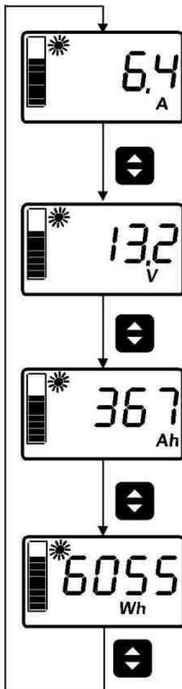
The measuring and display values of the solar installation are scrolled forward via button 1 (left).
