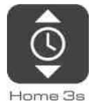
Button 2: Switches the time and thermometer displays, programs the home screen (3 s)
