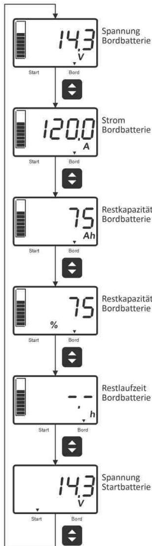
The measuring and display values of the battery computer functions are scrolled forward via button 1 (left)
