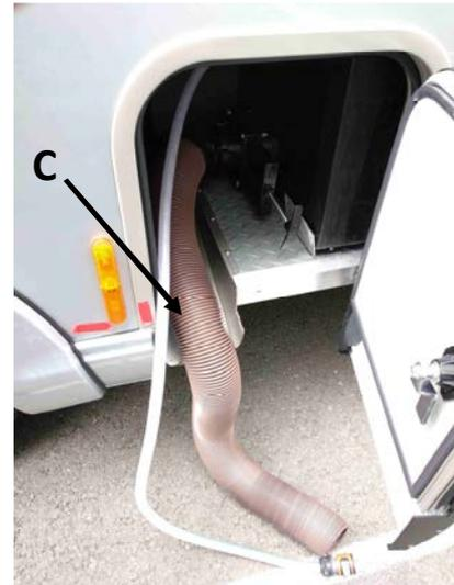
The dejection tank should be emptied and flushed thoroughly after each trip. Please make sure that the tank is completely empty especially if the motorhome is not used during the winter months.
