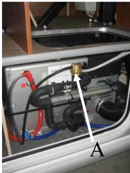
The heating system includes a water heater with the capacity of approx. 8.5 liters of fresh water. It is possible that air can accumulate in the pipes of the water heating. Please use venting screws on the radiators within the seating areas, kitchen and sleeping areas to release any air.
