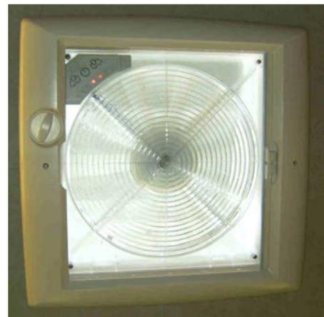
“Fiamma” roof lids with ventilator are opened by turning the knob. The ventilator sense of rotation can be controlled with the rocker switch.
