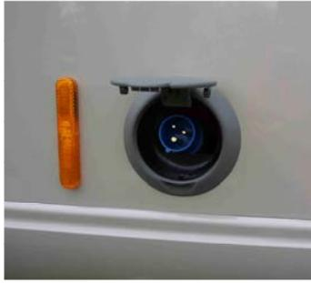
The self-retracting cable reel is behind a separate flap next to the central services unit. Pull out the power cable. Pull again lightly to trigger the self-retracting mechanism.
