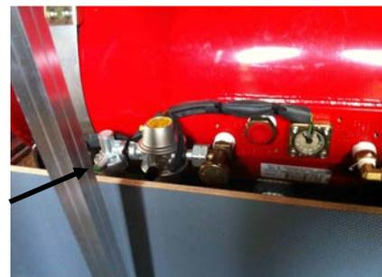
If there are gas bottles installed in addition to the gas tank, choose the gas source with the 3-way valve. The 3-way valve is installed near the gas distributor.
