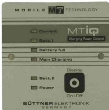
The "Display On/Off" button only switches the display off (e.g. night mode) or on. The operation of the charging boosters is not impacted).
