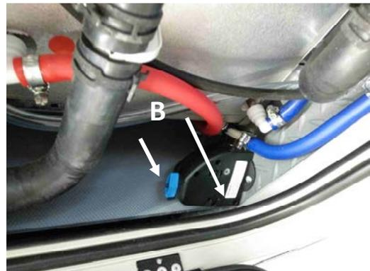
The temperature inside your motorhome should be at least + 6 °C. The valve will not close if any colder. If necessary, switch on the heating.
